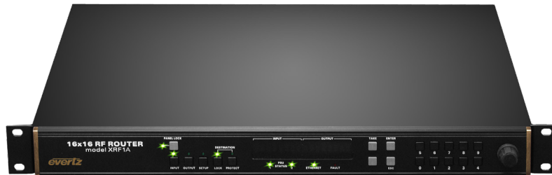
XRF1A with Local Control Panel (+LCP)
