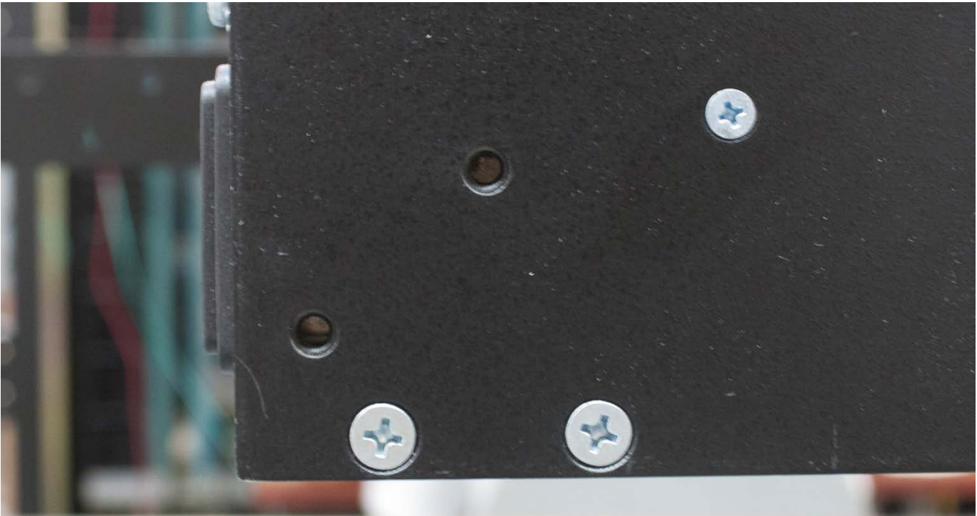
Figure 1-3: Holes Used to Attach the Metal Bar to the 7800FR
