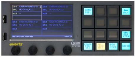
Figure 7-15: Selecting the "LOCK DST" Button
