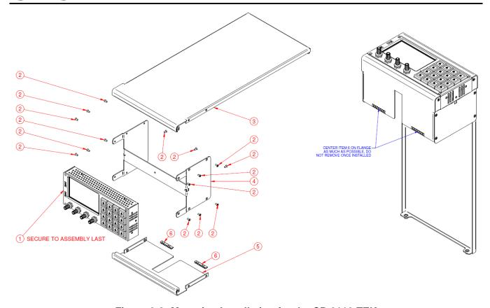
Figure 2-8: Mounting Installation for the CP-2116-TEK
