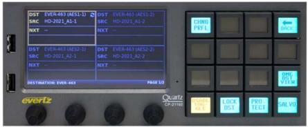
Figure 7-14: Selecting the "ENABLE TOGGLE" Button
