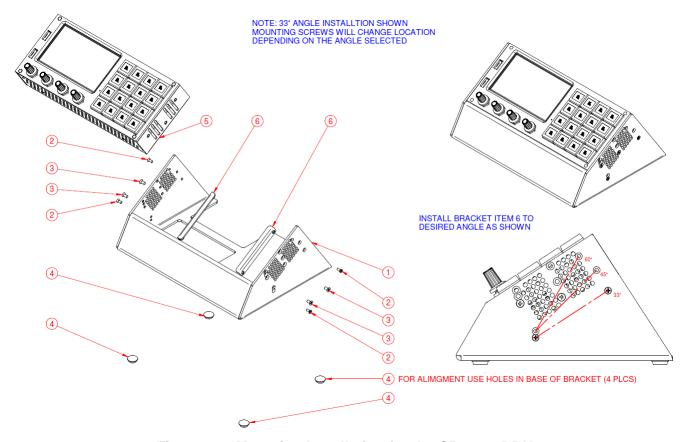
Figure 2-7: Mounting Installation for the CP-2116-DBK
