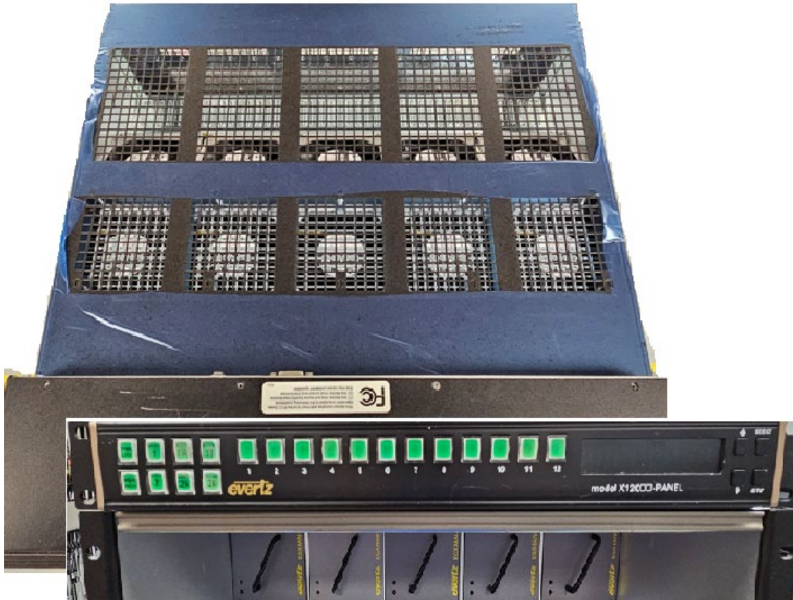
Figure 3-4: Shallow Panel not Blocking Venting Holes
