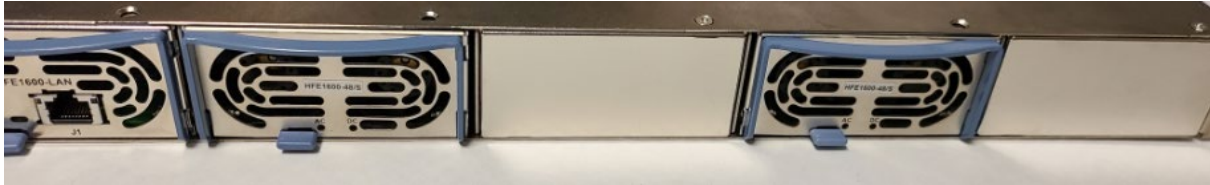
Figure 2-10: EQX-PS-FR-C Front View Partially Loaded with Blanks
