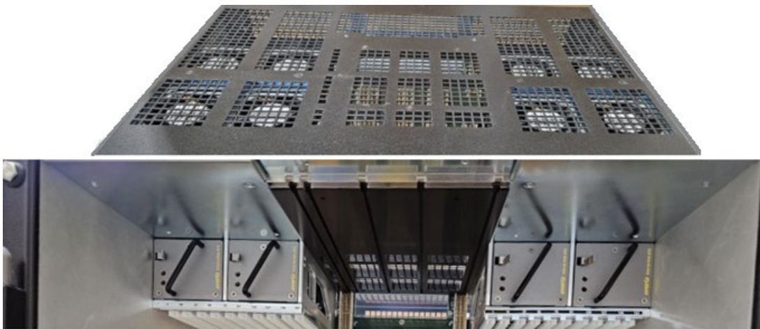
Figure 3-3: EQX10 & EQXUHD Frame Both Fans Vent Upwards
