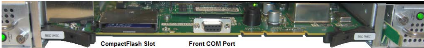
Figure 1-4: Front Panel Removed, CompactFlash Location
