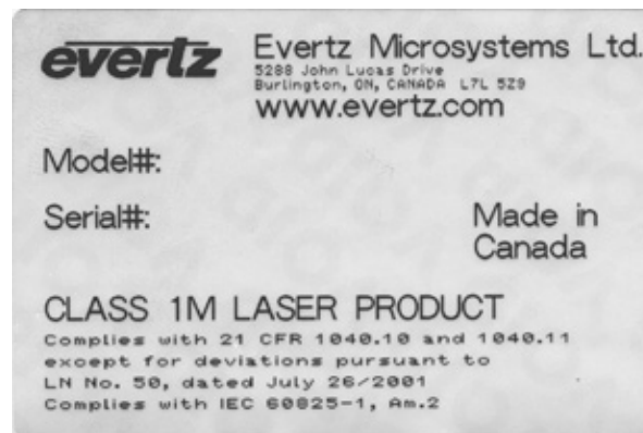
Figure 2-3: Reproduction of 7708LT Certification and Identification Label for Models that are Class 1M Laser Products
