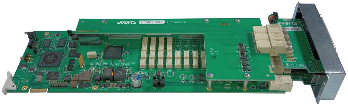
**Figure 1-1: 7800TR-32x24 with Accompanying Rear I/O Module (Rear plate)**
