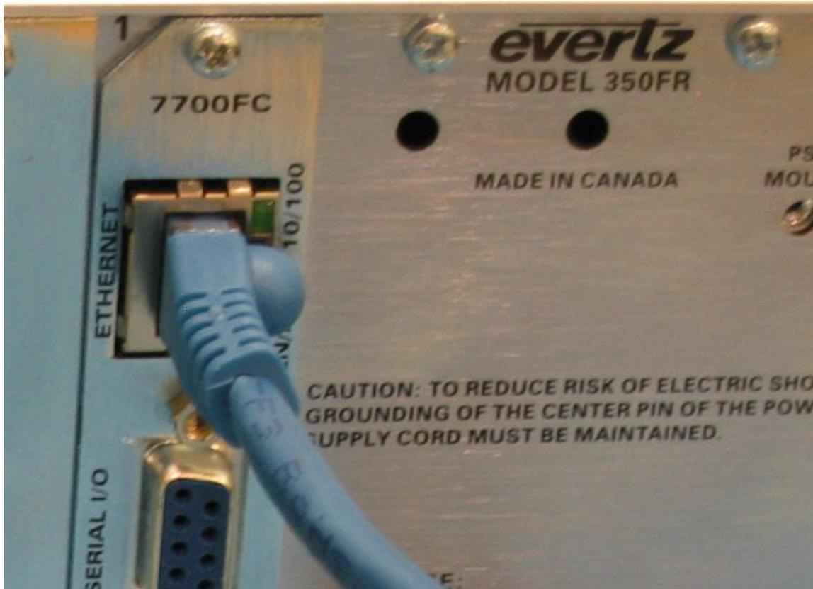
Figure 3-1: Connecting the 7700FC Frame Controller to the PC
