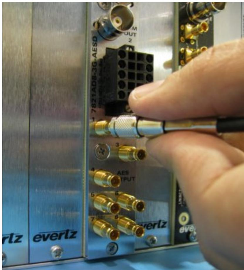
**Figure 3-4: Connecting to the AES Outputs of the 7821AD8-3G-AESD**
