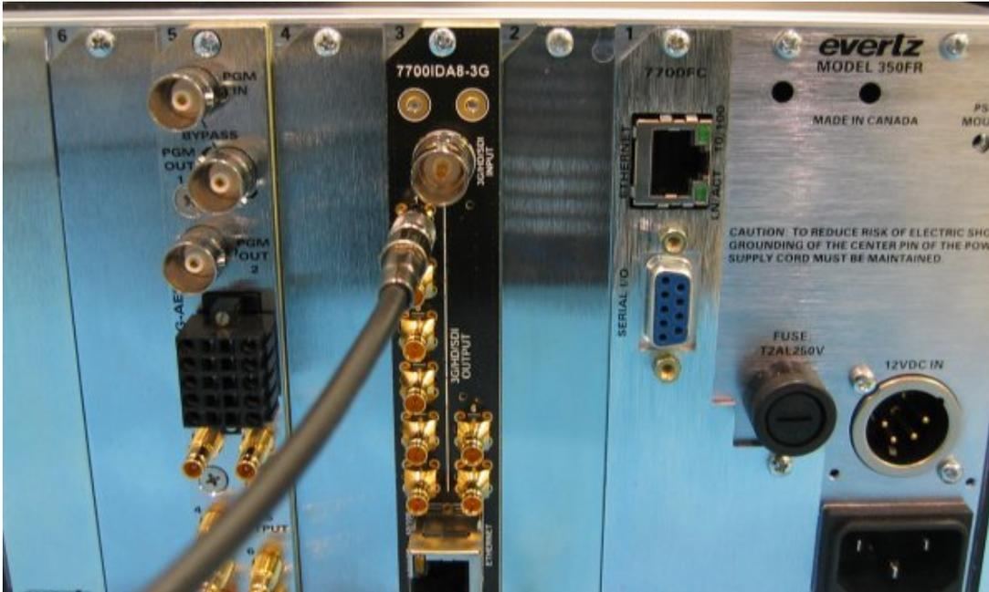
**Figure 3-2: Connecting the output of the 7800IDA8-3G+IG IntelliGain Processor**
