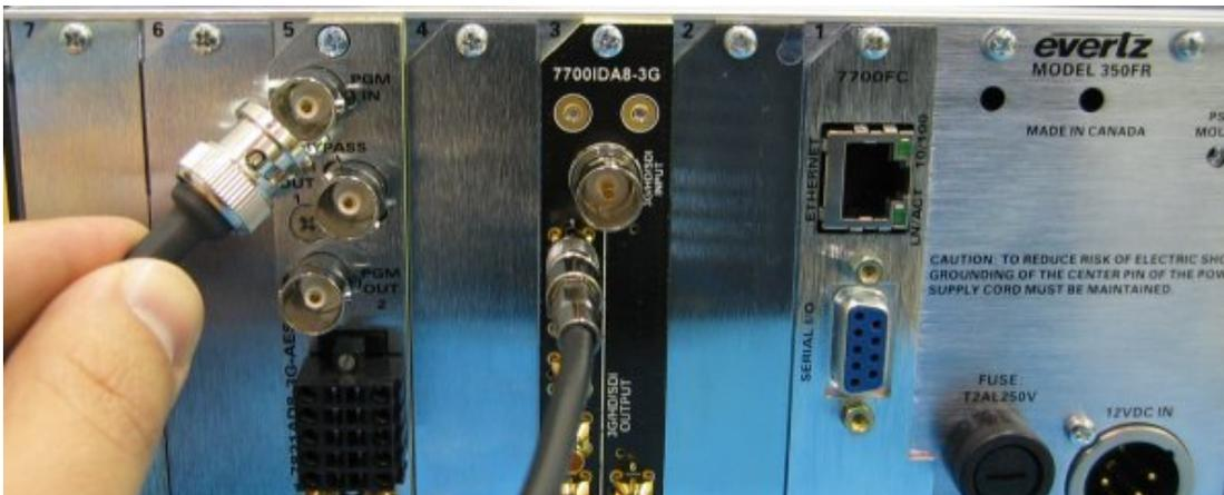
**Figure 3-3: Connecting the Input of the 7821AD8-3G-AESD Audio De-embedder**
