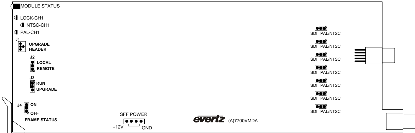
Figure 6-1: LED and Jumper Locations (Rev A)
