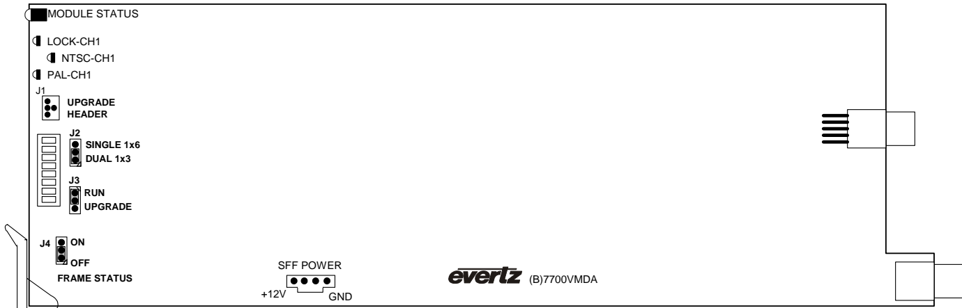
Figure 6-2: LED and Jumper Locations (Rev B)
