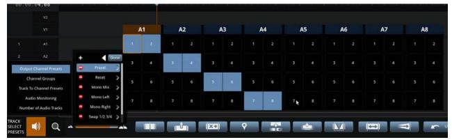
Figure 7-9: Creating a new Output Channel Preset
