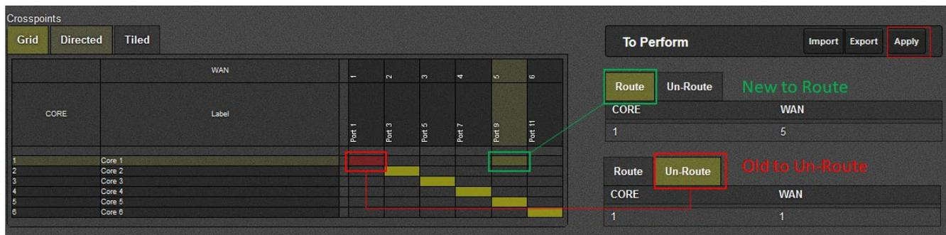
Figure 4-19 : WebEASY® - Link Aggregation\Grid View\To Perform in Grid
