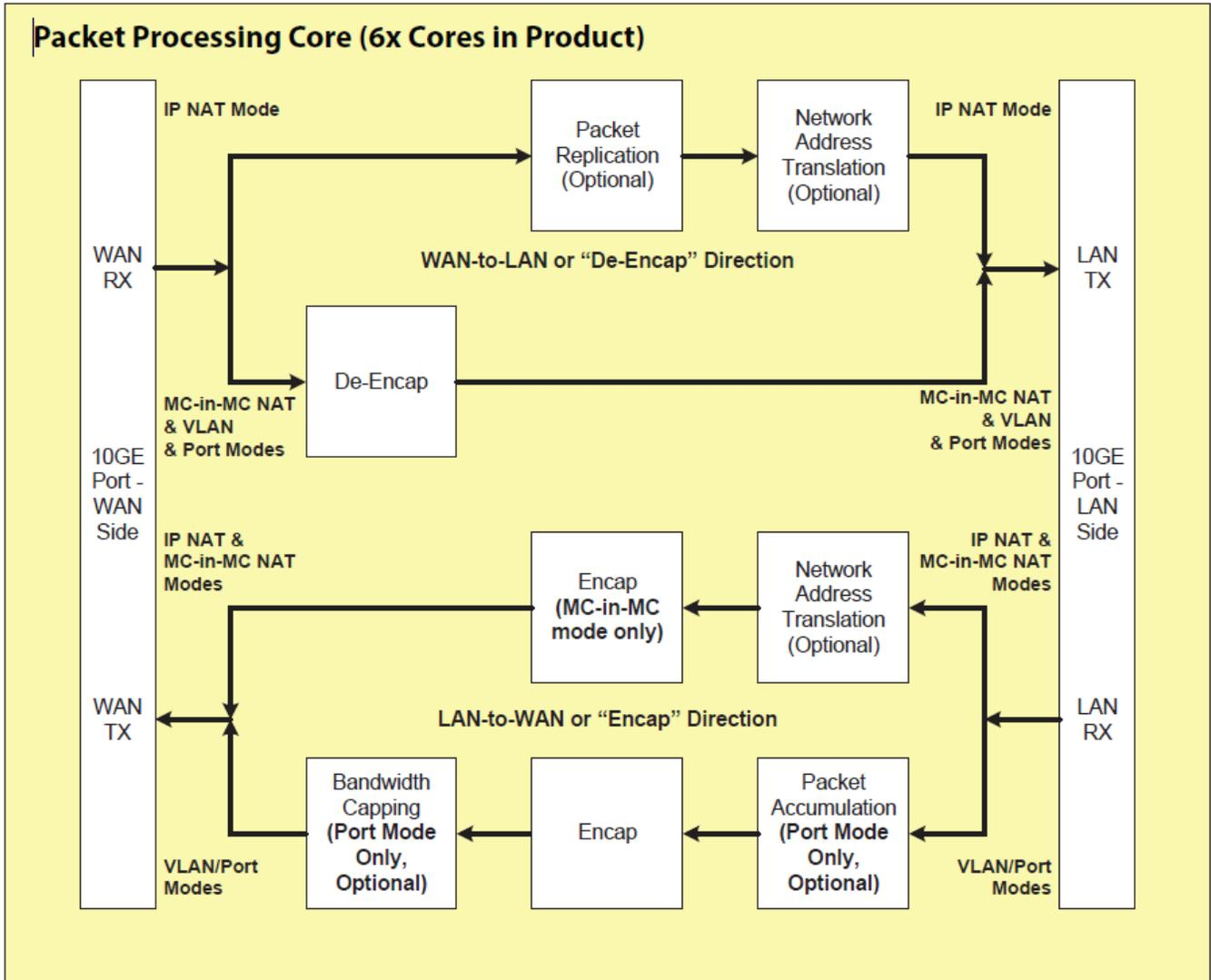
**Figure 1-1: Single NAT Core Block Diagram**
