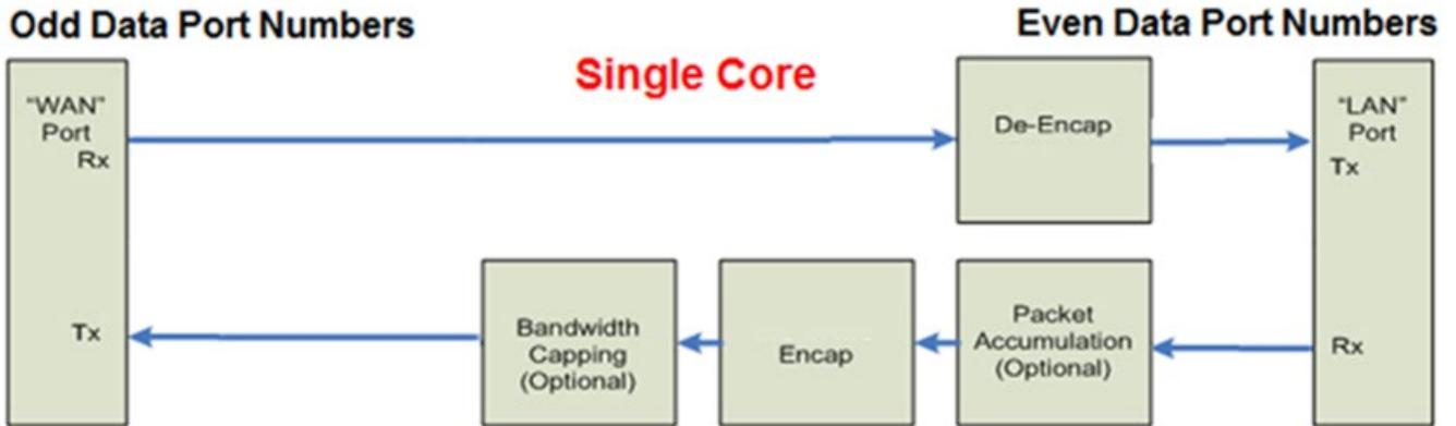
**Figure 4-6 : Port Based NAT Mode Block Diagram**
