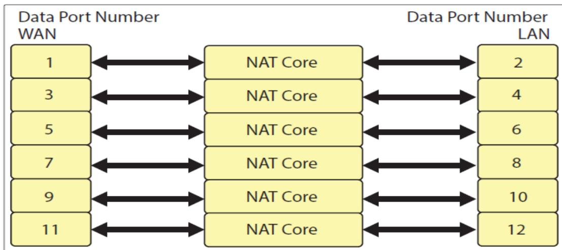
**Figure 1-2 : 570NAT-HW-X19 Core Mapping Block Diagram**
