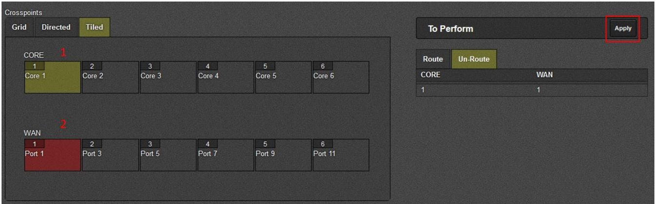
**Figure 4-28 : WebEASY® - Link Aggregation\Directed View\Removing Links in Tiled**
