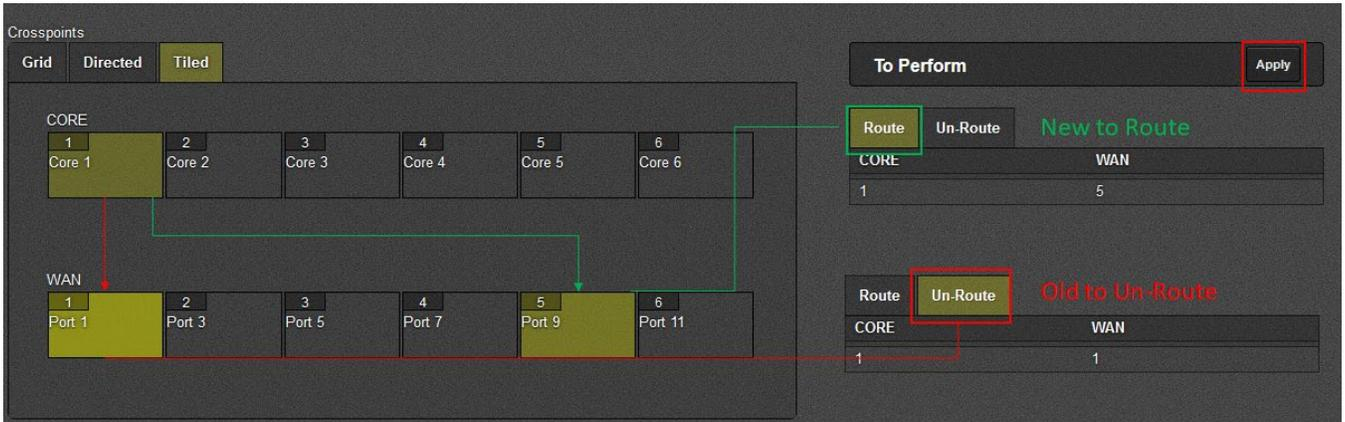
**Figure 4-27 : WebEASY® - Link Aggregation\Tiled View\Linking in Tiled**
