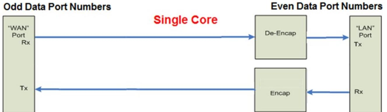
Figure 4-8 : VLAN Based NAT Mode Block Diagram
