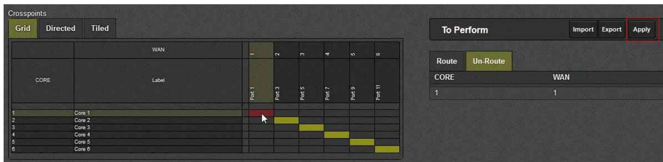
Figure 4-20 : WebEASY® - Link Aggregation\Grid View\Removing Links in Grid
