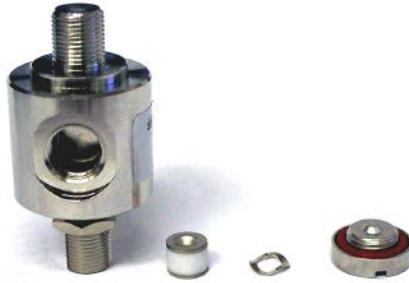
Figure 3-3: 2400ODU Lightning Suppressor – Disassembled, Gas Tube and Spring Washer Removed
