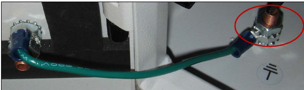
Figure 2-5: 2400ODU Enclosure Ground Stud
