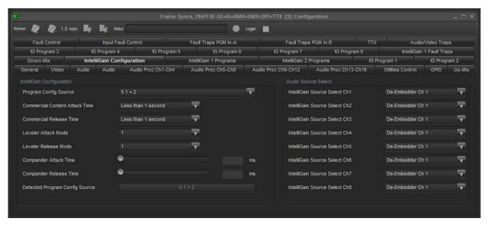
Figure 5-9: IntelliGain Configuration Tab
