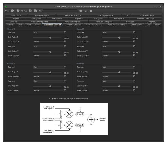
Figure 5-4: Audio Proc Ch1-Ch4 Tab
