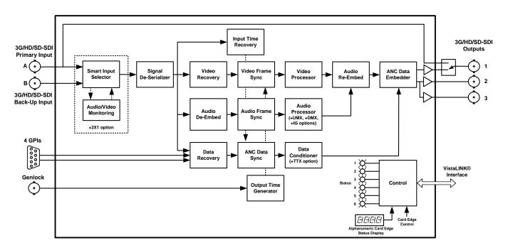
Figure 1-1: 7847FSE Frame Synchronizer Block Diagram
