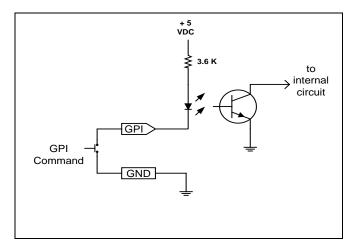
Figure 2-2: GPI Input Circuitry
