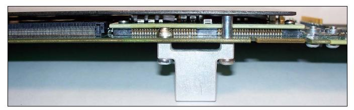
Figure 6-2: Slot Blocker
