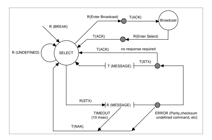
Figure 4-1: Communications Protocol State Diagram
