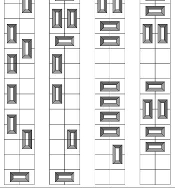
Figure 5-1: Jumper Settings for Serial Port Configurations
