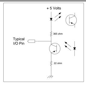
Figure 2-2: Typical GPIO Circuitry
